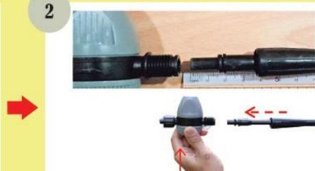
2 Ganti pengatur tekanan jika rosak Replace pressure regulator if faulty
